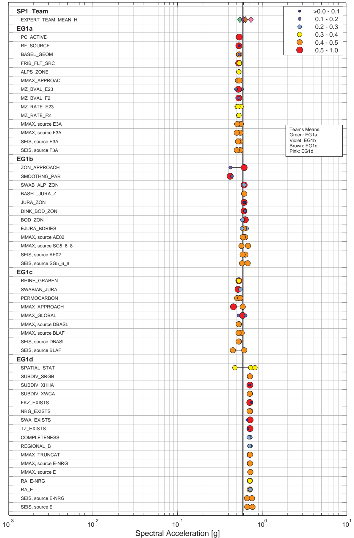
Figure 4.16.6: Leibstadt, horizontal component, rock, sensitivity histogram for SP1, 100 Hz, 1E-06.
