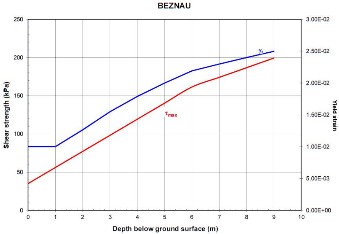
Figure I-8.4: KKB - Shear strength and yield strain versus depth.
